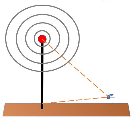
The antenna at the base station is assumed to be isotropic and has power 1 [unit Watt]. We consider the signal traveling in 3D surface and the cell tower is 21 meters above the ground.
